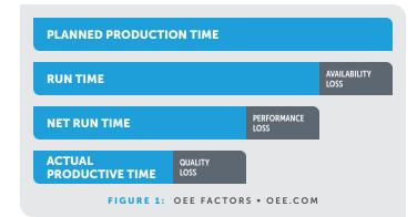
As illustrated in **Figure 1**, to achieve 100% OEE requires the Actual Production Time to equal the Planned Production Time, which means 100% Quality (only good labeled products), 100% Performance (labeling as fast as possible) and 100% Availability (no stopping). Despite the stringent quality standards in label application and appearance, industry trends are driving Personal Care and Household product manufacturers to take more notice of their productivity.
